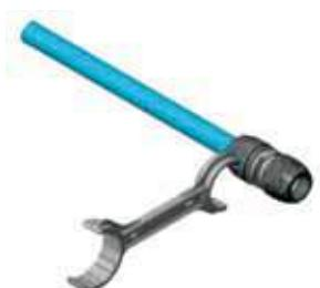
Fully tighten the ring nut and then rotate up to 180° maximum using a pin wrench of suitable size
