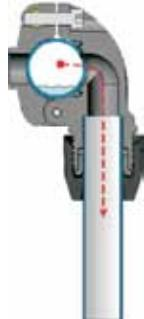
From the picture you can see that the air intake is positioned above the lowered level of the condensation
